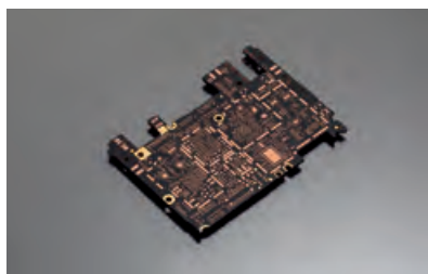
FWSS® (Free via stacked up structure)
